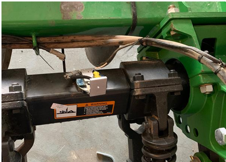
Figure 19: Work switch mounting location
