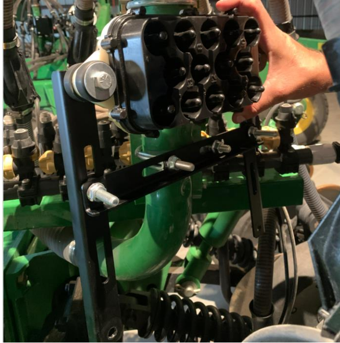
Figure 11: ECU installed on a tower (horizontal installation)
