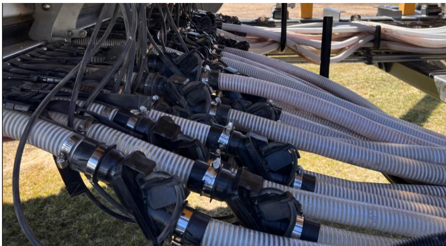
Figure 4: Installing flow sensors on on-frame tanks
