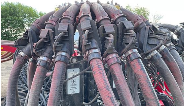
Figure 2: Flow sensor installation location
