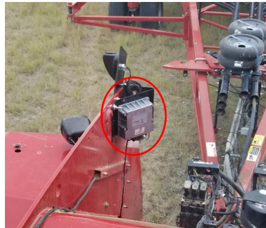
Example tow-behind mounting location (on the frame)
