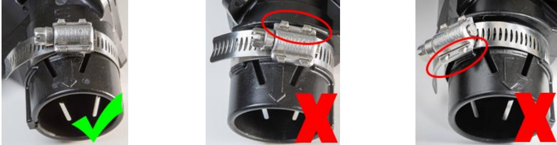
Figure 5: Correctly placing the hose clamps
