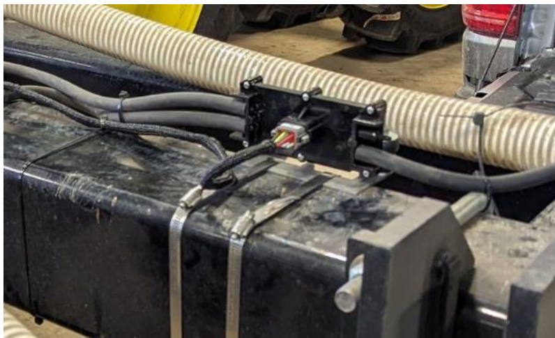
Figure 12: Auditory tube zip tied to the frame
