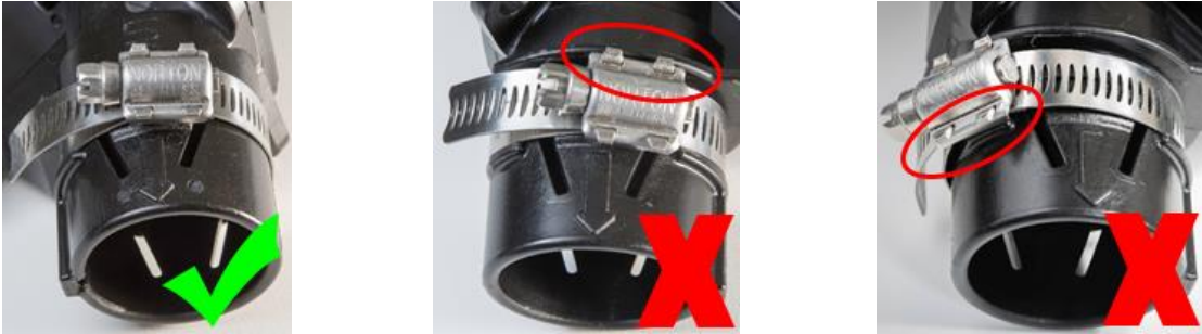
Figure 4: Correctly placing the hose clamps
