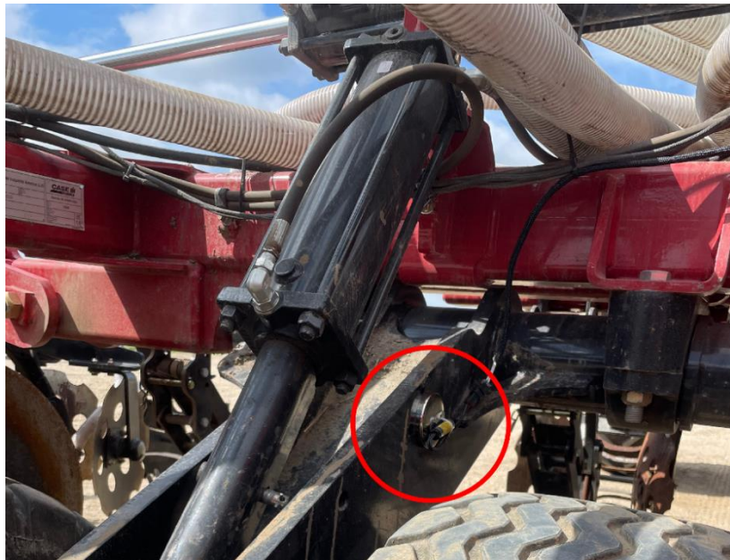
Figure 14: Work switch mounting location
