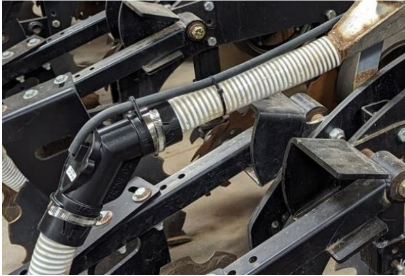
Figure 11: Auditory tube zip tied to the hose
