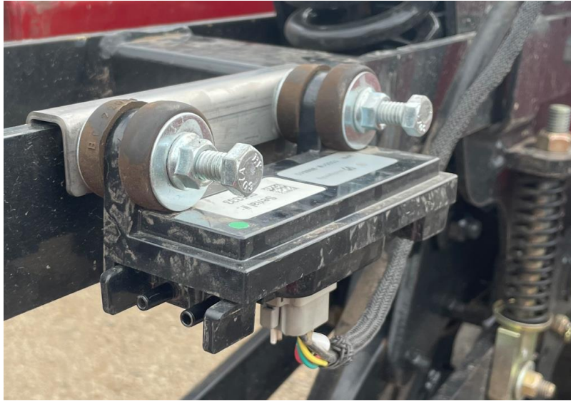
Figure 9: Installed C-channel bracket ECU
