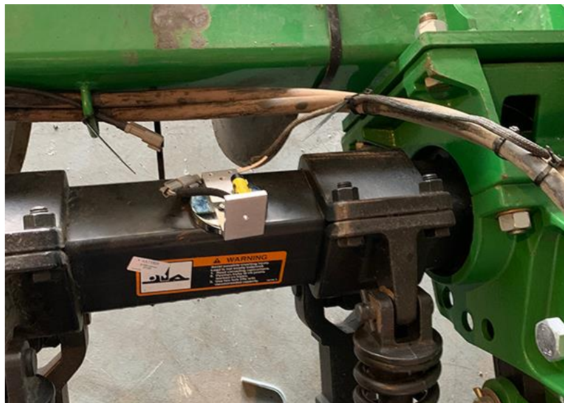
Figure 16: Work switch mounting location
