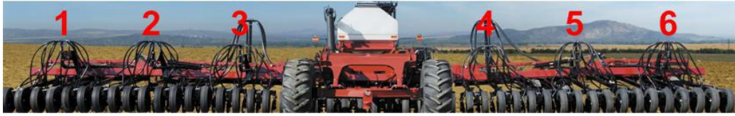
Figure 11: Installing the ECUs from left to right
