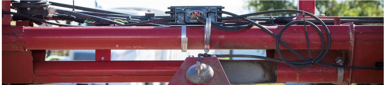
Figure 6: Auditory tubes connected to an ECU
