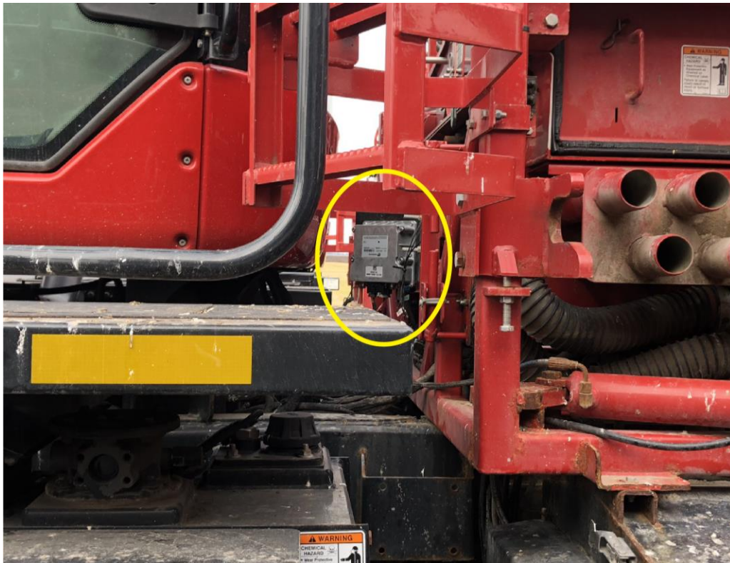
Figure 7: Gateway mounting location
