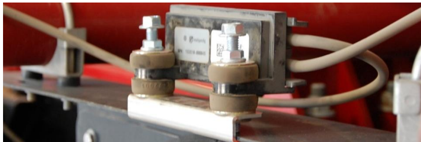
Figure 5: Installed C-channel bracket ECU
