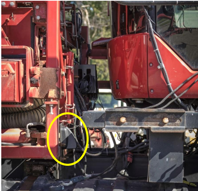
Figure 10: Wi-Fi antenna mounting location
