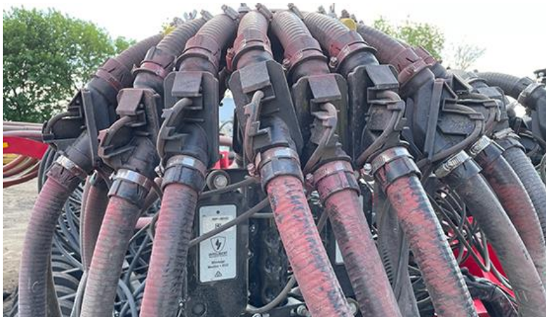
Figure 2: Flow sensor installation location
