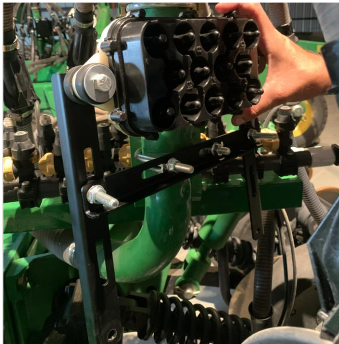
Figure 10: ECU installed on a tower (horizontal installation)
