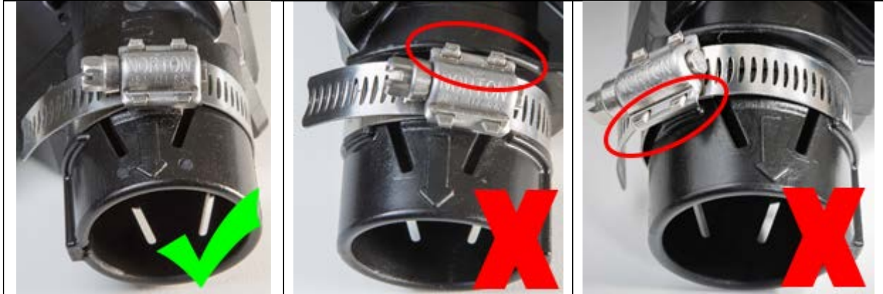
Figure 6: Correctly placing the hose clamps
