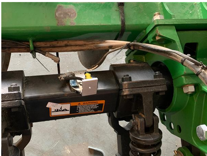
Figure 16: Work switch mounting location
