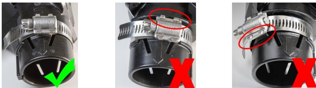
Figure 4: Correctly placing the hose clamps
