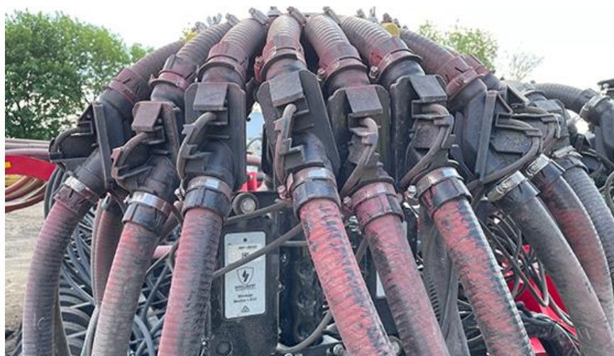
Figure 2: Flow sensor installation location
