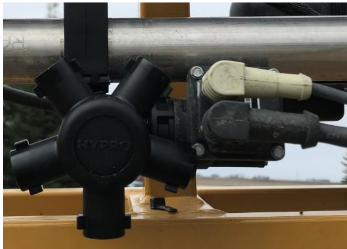
Nozzle body with ProStop-E valve
