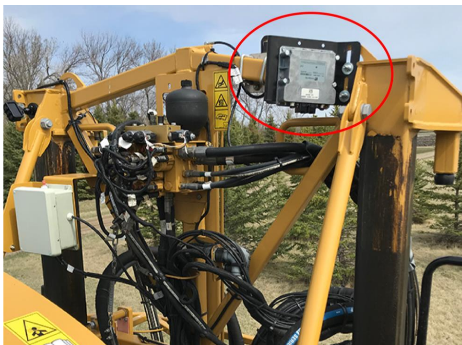
Figure 7: Gateway mounting location
