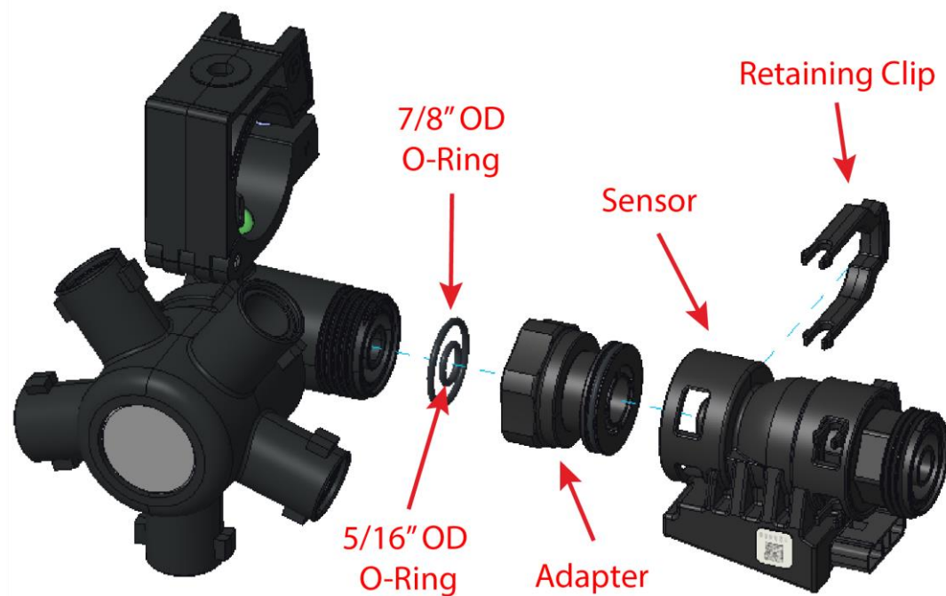
Figure 1: Flow sensor installation overview
