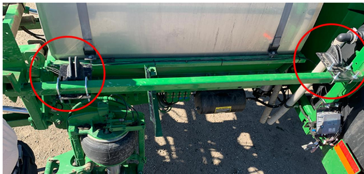
Figure 9: Antenna mounting location
