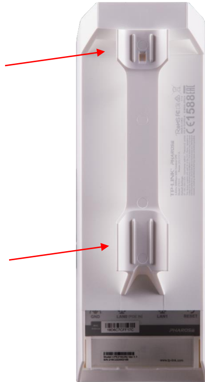
Figure 21: Apply the gaskets to the feet of the access point
