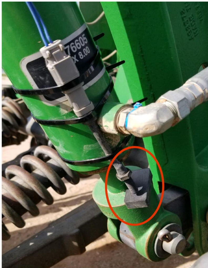
Figure 16: Installing a proximity switch on an implement with no existing work switch
