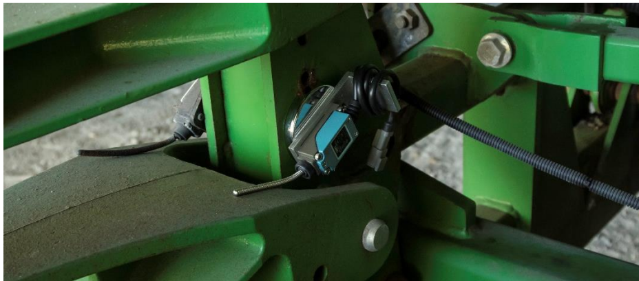
Figure 15: Mounting location for whisker switch (900000-000001)
