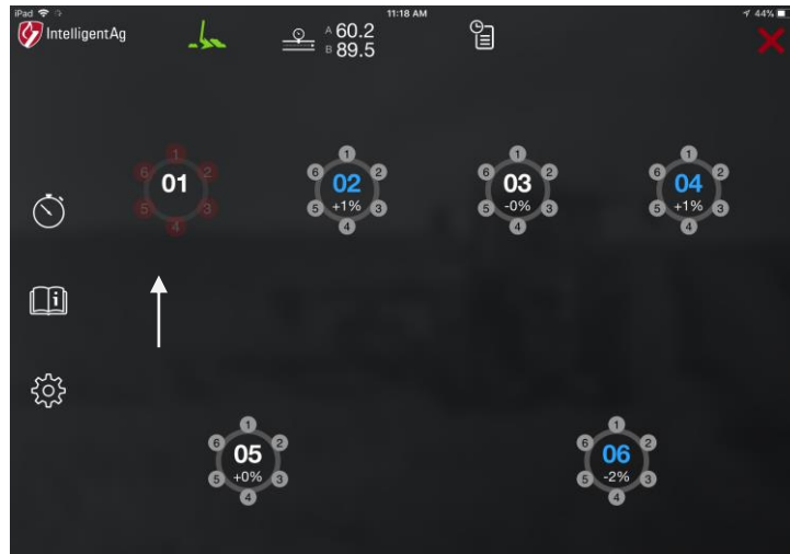
Figure 19: Blockage screen showing a manifold not seeding due to section control
