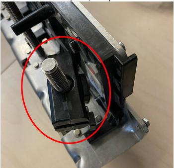
3. Using a 5.5 mm socket, ratchet and extension, remove the four 5.5 mm screws, rubber washer, and the two stainless steel plates from the face of the motor. Then, remove the motor from the motor mount.
