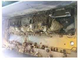
Intelligent Ag implemented improvements to the motor in spring 2020, including a corrosion resistant coating; **however**, the best protection against severe corrosion is the proper cleaning and maintenance of unit. This will help ensure motor corrosion is minimal and reduces the likelihood that a replacement will be needed next season.
