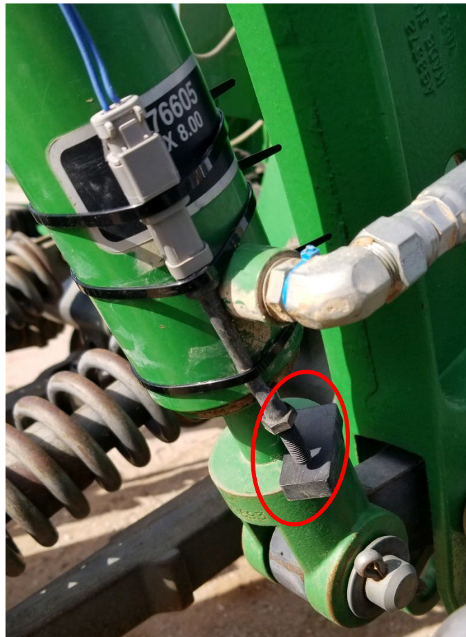
Figure 18: Installing the proximity switch
