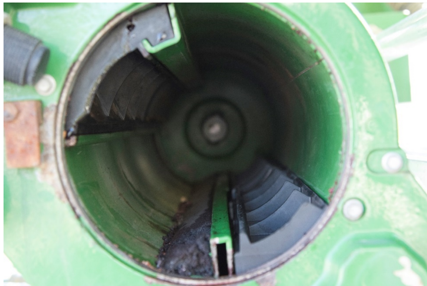
Figure 7: Inserting meter housing dividers
