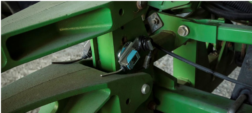
Figure 16: Installing the whisker switch
