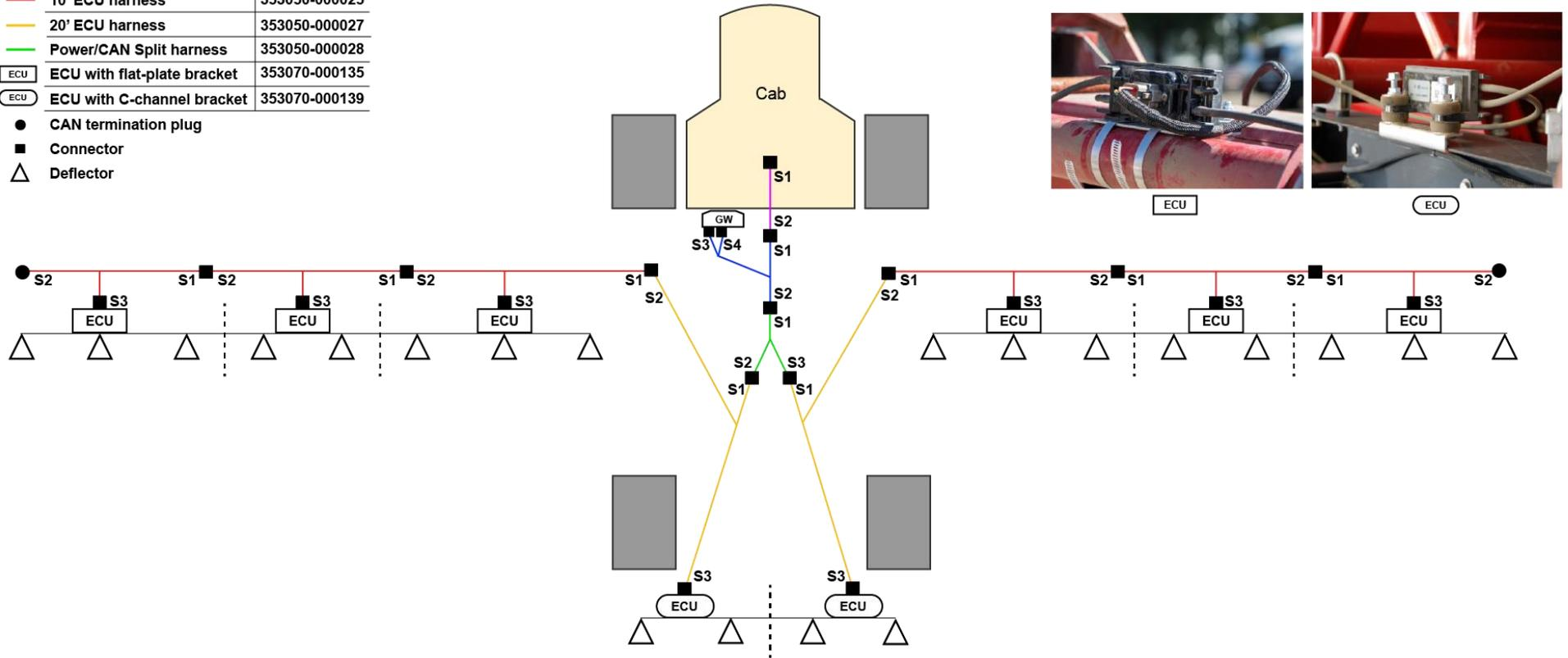
**TIP:** Start with harnessing on the leftmost and rightmost side of the booms and work toward the center. Then, work on harnessing toward the cab.
