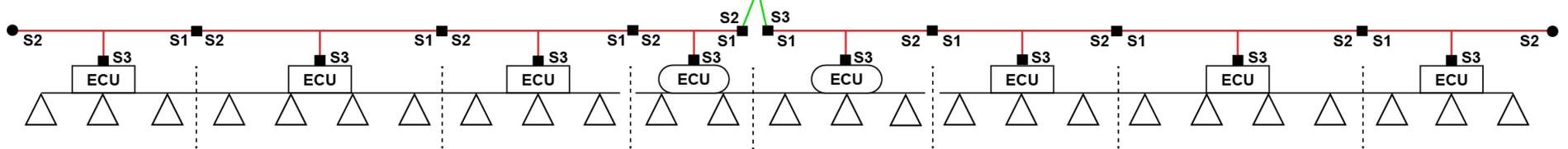
**TIP:** Start with harnessing on the leftmost and rightmost side of the booms and work toward the center. Then, work on harnessing toward the cab.
