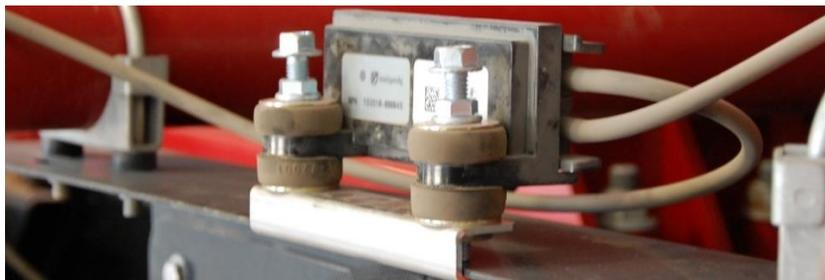
**Figure 5: Installed C-channel bracket ECU**
