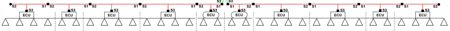
**TIP:** Start with harnessing on the leftmost and rightmost side of the booms and work toward the center. Then, work on harnessing toward the cab.
