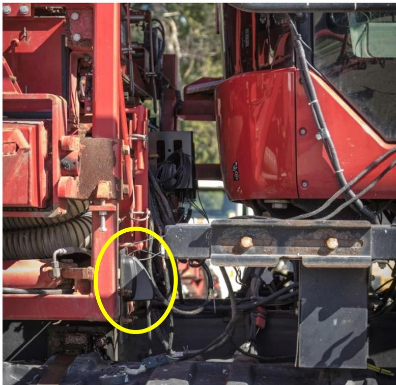
Figure 10: Wi-Fi antenna mounting location
