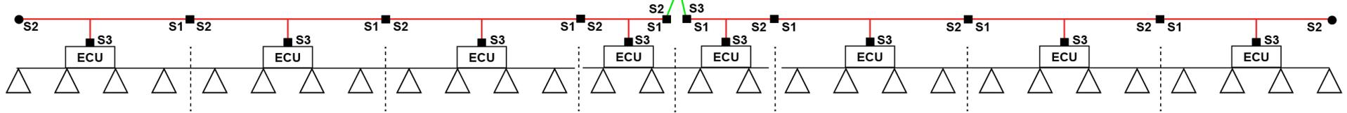
**TIP:** Start with harnessing on the leftmost and rightmost side of the booms and work toward the center. Then, work on harnessing toward the cab.
