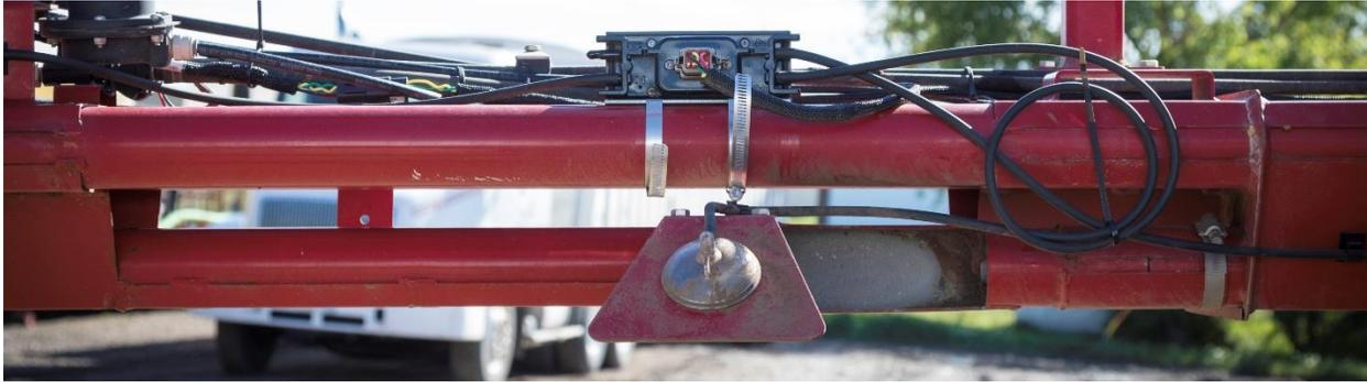
Figure 6: Auditory tubes connected to an ECU
